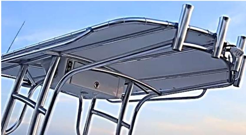
*Deluxe Soft T-Top option comes with the Sport package. The T-Top switch turns on the blue courtesy light. The SPREADER switch operates the front and back spreader light.*
