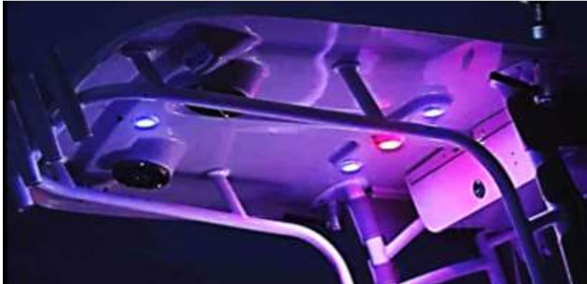
*Fiberglass T-Top option comes with the Platinum package. The T-Top switch turns on the 3 blue courtesy lights. The SPREADER switch operates the 2 back spreader lights and the front spreader light. The switch on the map light may be turned one way for a red or the other way for a white light.*
